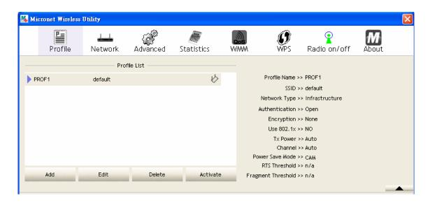
When a profile is selected and click on 'Activate' button, an icon will be displayed in front of the profile to show that the connection has failed. When the connection is successfully established, an icon will be displayed.
